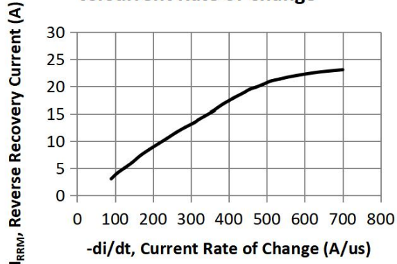
FIG.5 Reverse Recover Current vs. Current Rate of Change
