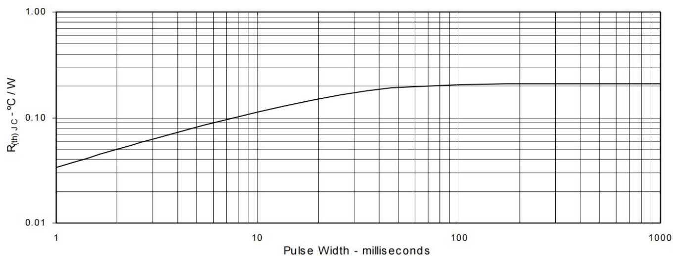
Fig 7: Maximum Transient Thermal Resistance
