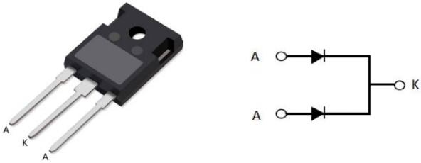
Package view and circuit symbol
